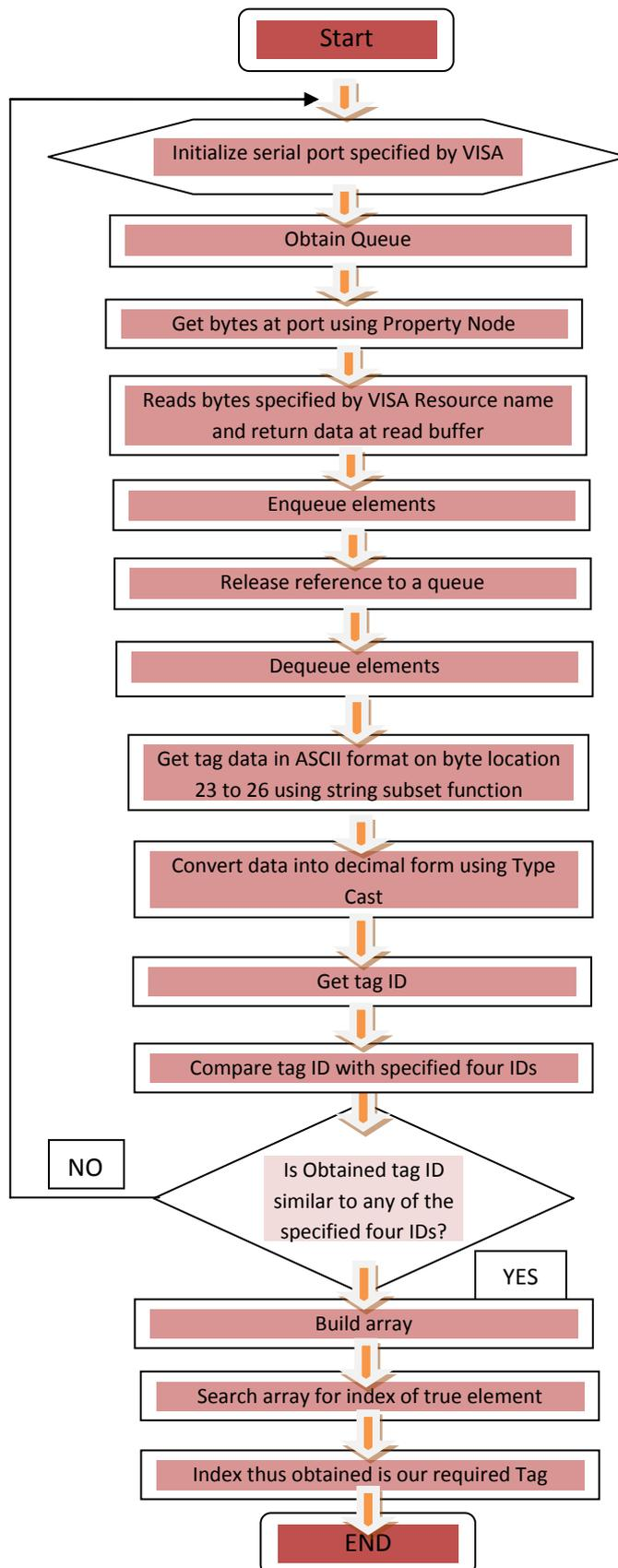
Figure 5. A flowchart showing sequence of tag detection events
