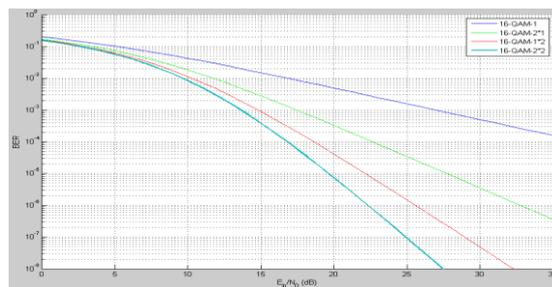
**Fig.9: SNR Vs BER performance analysis in WiMAX networks for 16-QAM modulation**
