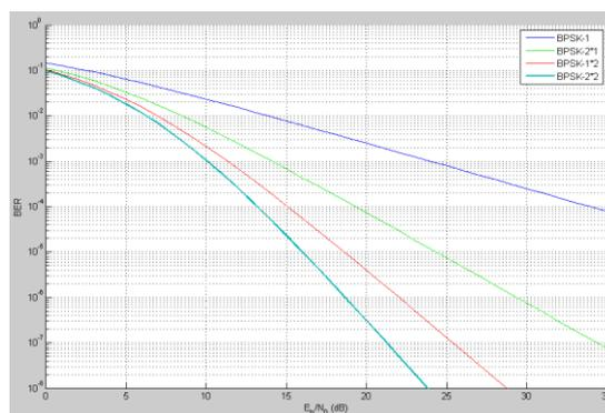
**Fig. 7: SNR Vs BER performance analysis in Wi-MAX networks for BPSK modulation**
