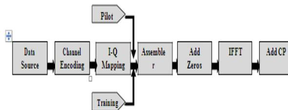
**Fig.5: Transmitter of the Wi-MAX system**
