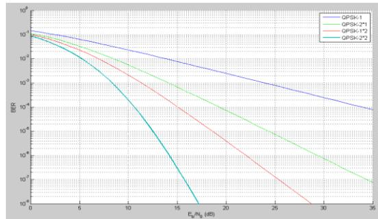
**Fig.8: SNR Vs BER performance analysis in Wi-MAX networks for QPSK modulation**
