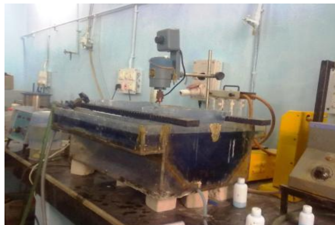
Figure 4. Experimental Lab scale ECAR reactor
