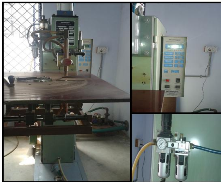
Figure 1: Resistance Spot Welding machine & its components
