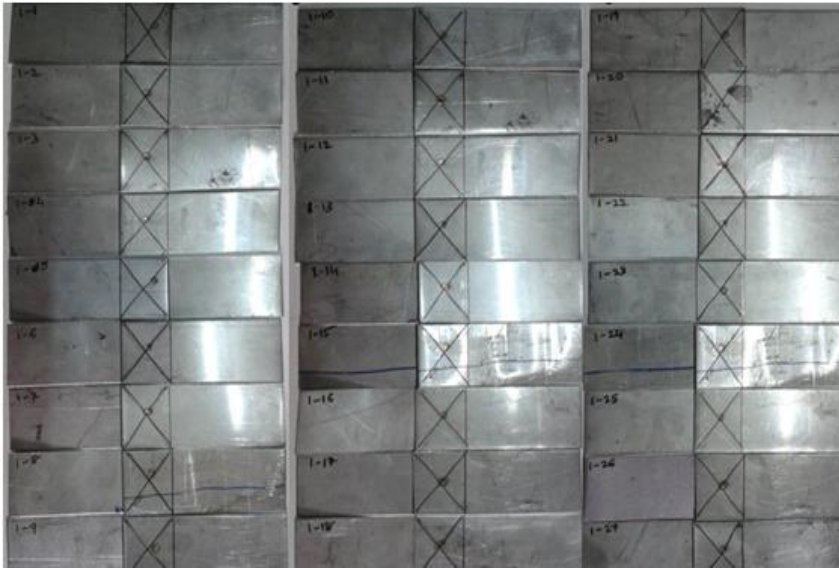
Figure 3: Specimens of Spot welded for SS304
