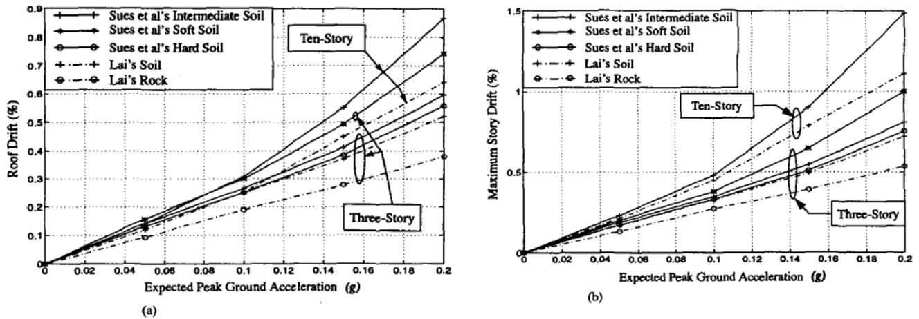
Figure 1: Expected drift levels for different ground accelerations: (a) roof drift versus ground accelerations; (b) maximum storey drift versus ground accelerations
