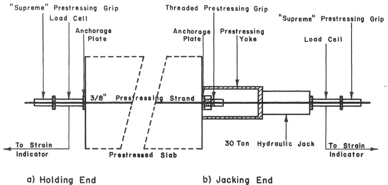
*Figure 2: Prestressing setup by holding and jacking ends*
