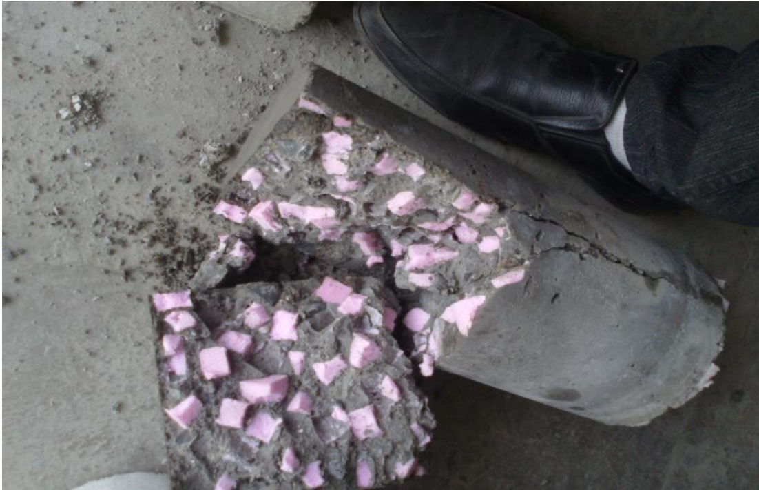
Figure 3.3 Cylinder split tensile strength test.
