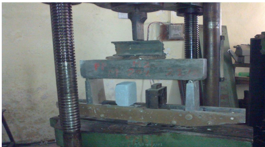
Figure 3.5 Experimental setup for Flexural Strength Test
