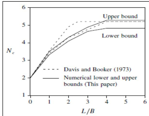
Fig 2.4: Lower and Upper Bound Bearing Capacity for Slopes
