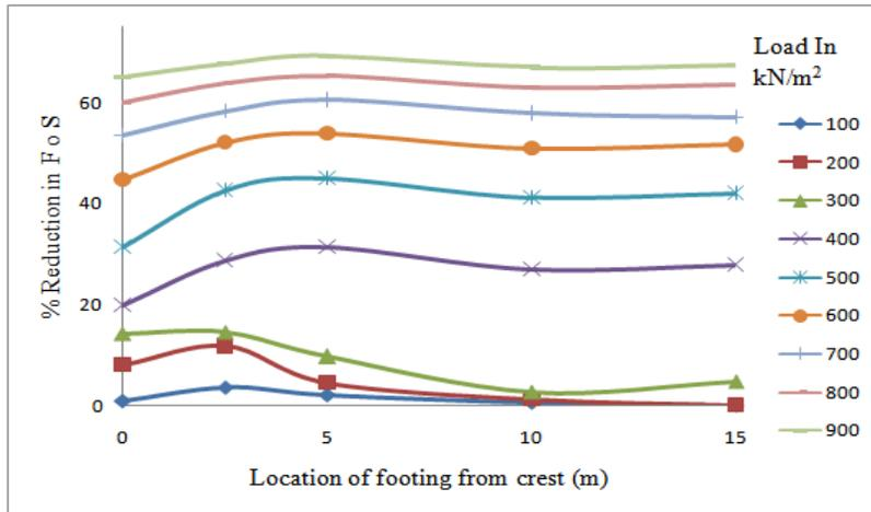
Fig 5.3: Percentage Reduction in Factors of Safety with Location of Footings for (1:2) Slope
