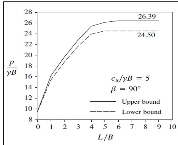
**Fig 2.2 Typical Upper and Lower Bound Results**
