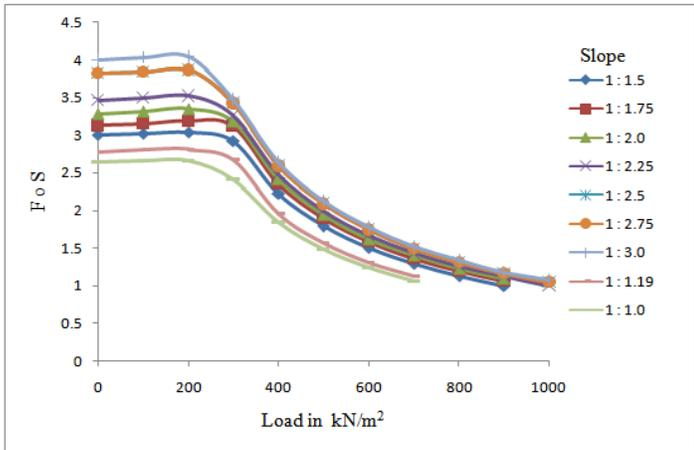
**Fig 4.5: Variation of Factors of Safety with Load at 15m Crest of Slope**
