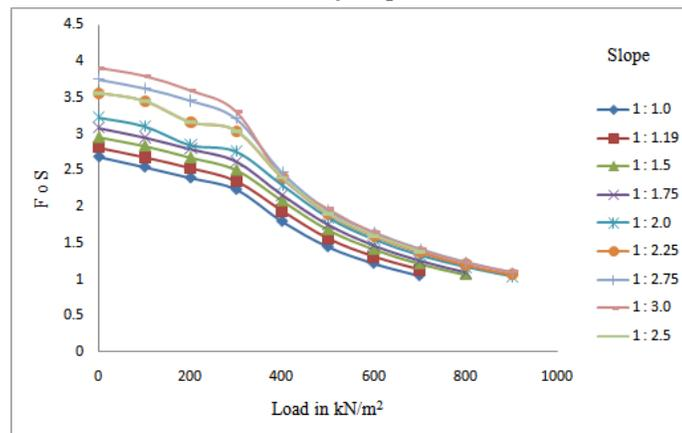
Fig 4.2: Variation of Factors of Safety with Load at 2.5m from Crest of Slope
