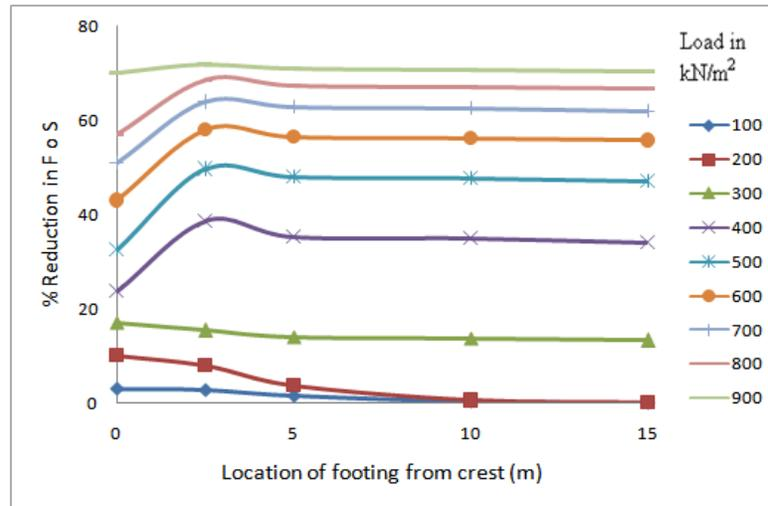
**Fig 5.5: Percentage Reduction in Factors of Safety with Location of Footings for (1:3) Slope**
