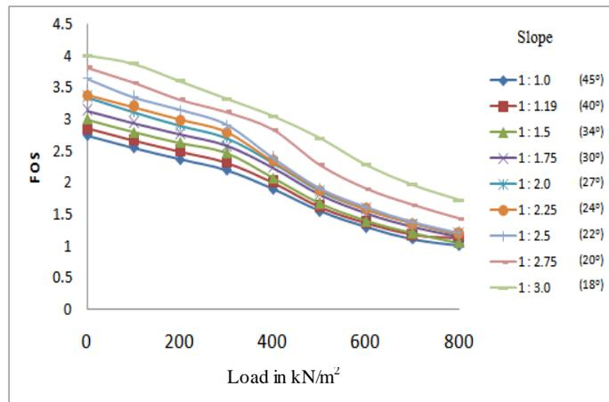
Fig 4.1: Variation of Factors of Safety with Load at Crest of Slope
