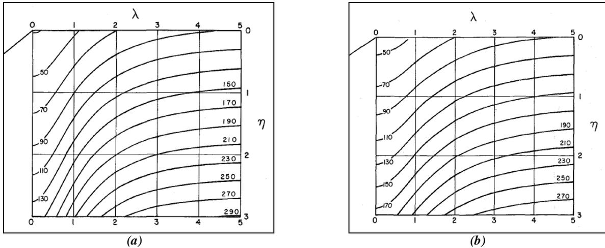
**Fig 2.1: Bearing Capacity Contours in Percentage for 1:2 (a) and 1:1.5(b) Slopes**
