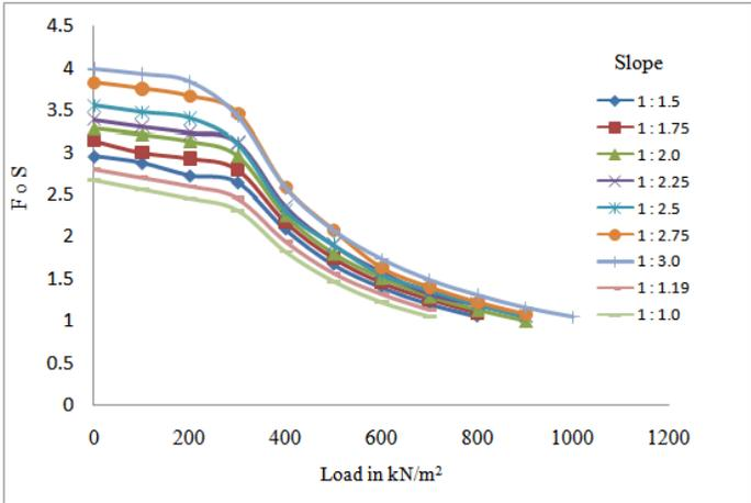
**Fig 4.3: Variation of Factors of Safety with Load at 5m from Crest of Slope**
