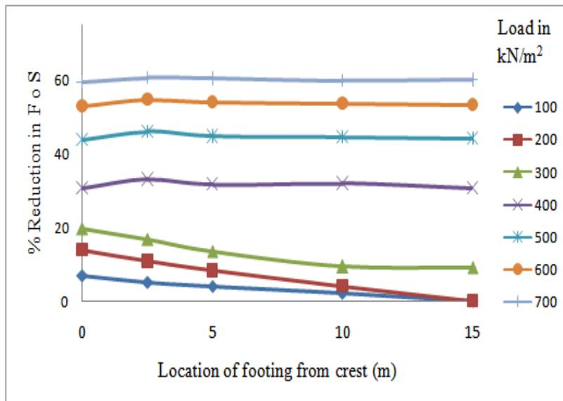
Fig 5.1: Percentage Reduction in Factors of Safety with Location of Footings for (1:1) Slope
