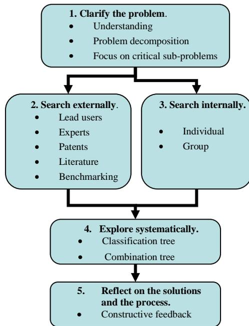
Fig 1. Flowchart of five-step concept generation method
