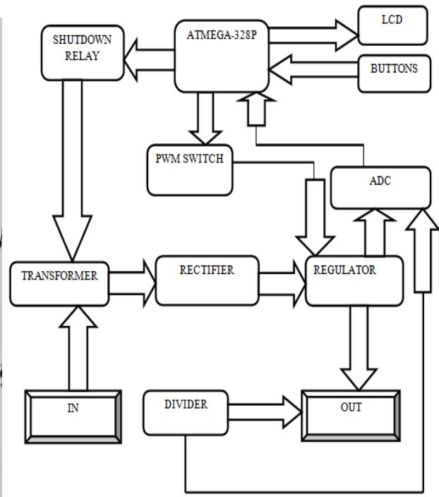
Figure 5-Detail block diagram of digitally controlled system
