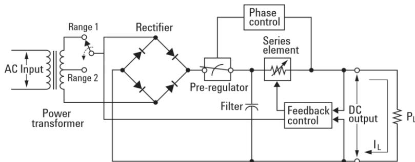
Figure- 6 a generic series element power supply
