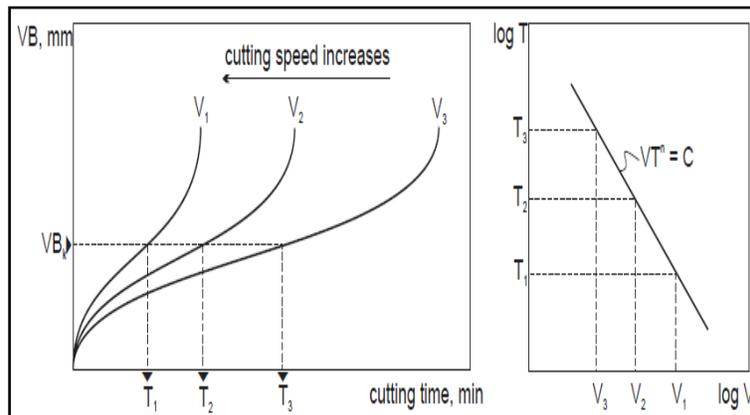
Fig 3 (Left) Effect of cutting speed on wear land width and tool life for three cutting speeds. (Right) Natural log-log plot of cutting speed versus tool life.
