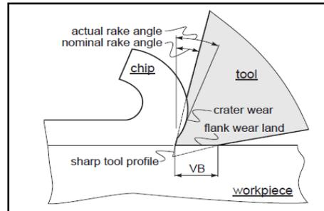
Fig1 Crater wear and Flank wear
