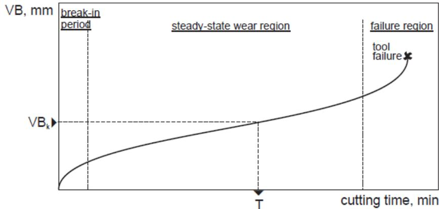
Fig 2 Flank wear as a function of cutting time. Tool life  $T$  is defined as the cutting time required for flank wear to reach the value of  $VB_k$
