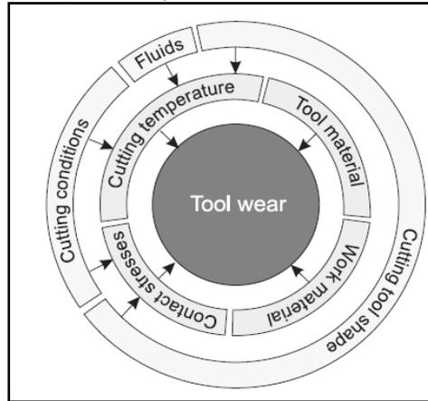
Fig 4 Cutting tool wear as a function of basic process parameters
