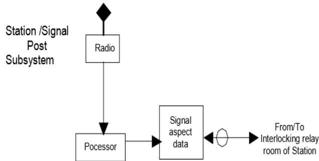
Fig 3. Station and Signal post subsystem of GPS based cab signalling
