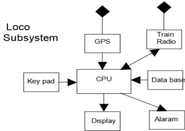
Fig 2. GPS based cab signalling for locomotive subsystem
