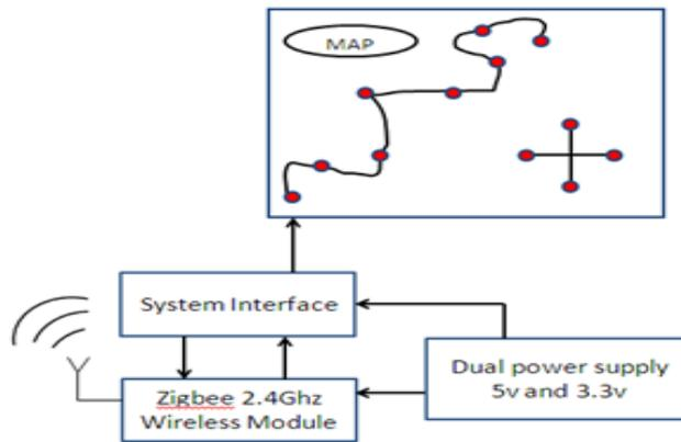
**Fig 7. Block diagram of monitoring unit**
