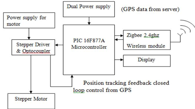
**Fig 6. Block diagram of the project**
