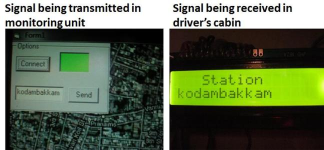
**Fig 10. Display image in the driver's cabin**
