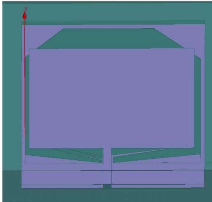
Fig1.UWB printed Slot antenna design using HFSS with dielectric constant ( $\epsilon_r$ ) = 3.52
