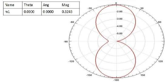
Fig3. Shows Gain of UWB slot antenna using dielectric substrate resonated at 2.5GHz with  $\phi (\varphi) = 0\text{deg}$  .
