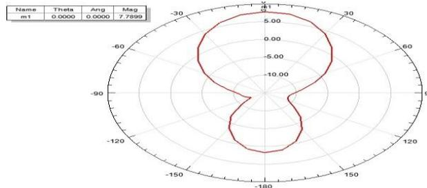
Fig4. Shows Gain of UWB slot antenna using dielectric substrate resonated at 3.5GHz ( $\epsilon_r=3.38$ ).
