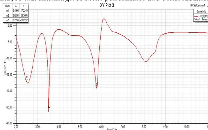
Fig2.Return loss of UWB slot antenna using dielectric substrate resonated at 2.5 GHz ( $\epsilon_r$  = 3.52)
