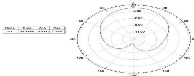
Fig5. Radiation pattern plot shows electric field variation with respect to theta values.
