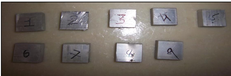
Figure 1 Specimens after Machining for AL-6351
