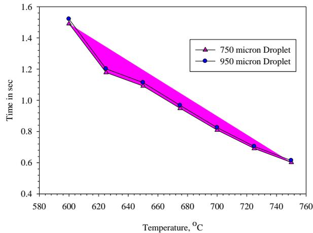
**Figure 8 Droplet diameter variations in Diesel at different temperatures**
