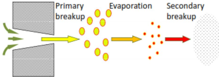
*Figure 1 Stages of droplet ignition of fuel*
