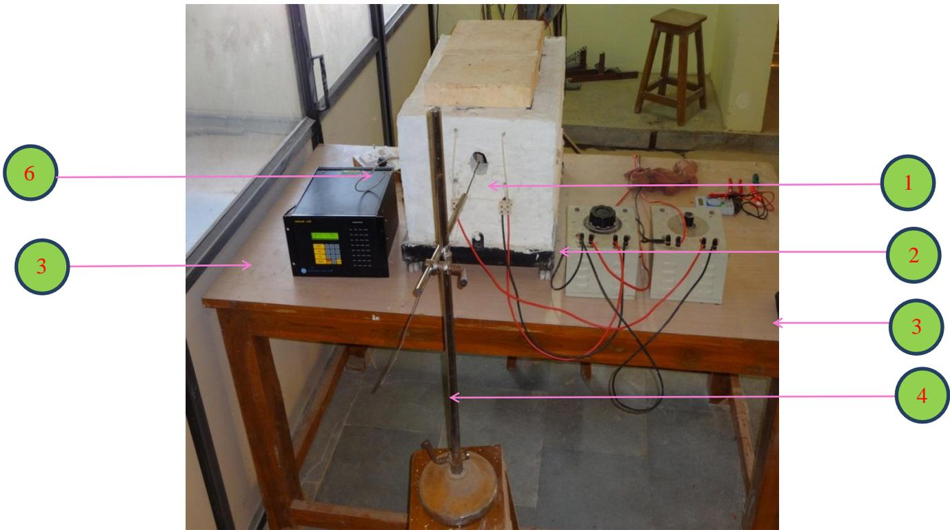
1. Opening Port (Diameter of 50 mm); 2. Combustion Chamber; 3. Kanthal Wire Wounded Heater (4 Numbers); 4. Windows (140x50mm); 5. Firebricks 6. Thermocouple (2 Numbers).
