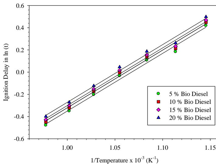
Figure 10 Ignition delay curve of blends of Bio-Diesel as a function of reciprocal of temperature (BD 5 to BD 20)
