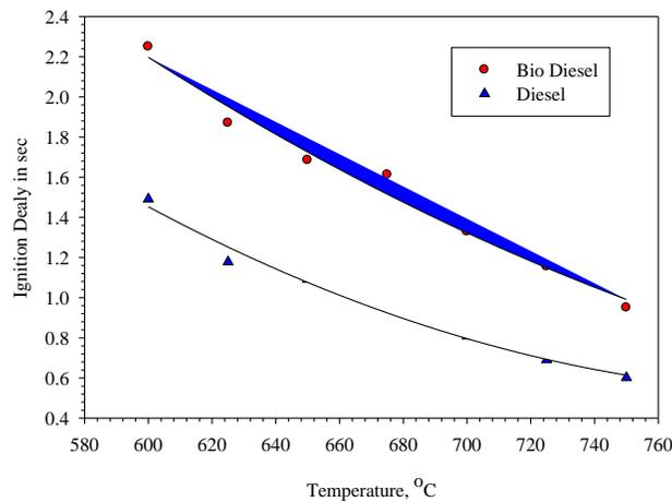
Figure 5 Ignition delay of Diesel and Bio-Diesel fuel at different temperatures
