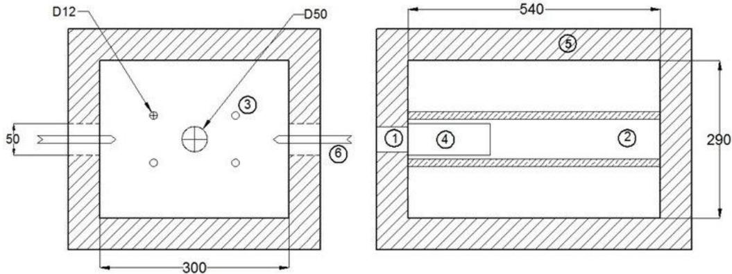
1. Opening Port (Diameter of 50 mm); 2. Combustion Chamber; 3. Kanthal Wire Wounded Heater (4 Numbers); 4. Windows (140x50mm); 5. Firebricks 6. Thermocouple (2 Numbers).
