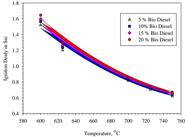
Figure 6 Ignition delays of blends of Diesel and Bio-Diesel fuel at different temperatures (5-20% of Bio-Diesel)
