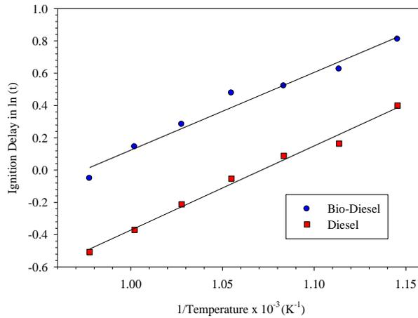
Figure 9 Ignition delay curves of Diesel and Bio-Diesel as a function of reciprocal of temperature
