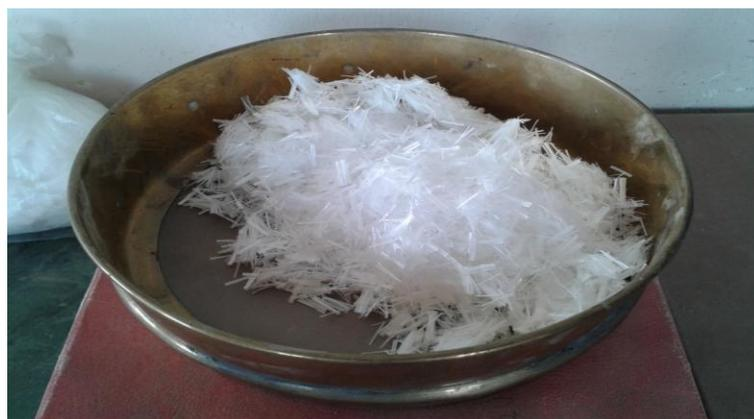
*Figure 3: Polypropylene fiber*
