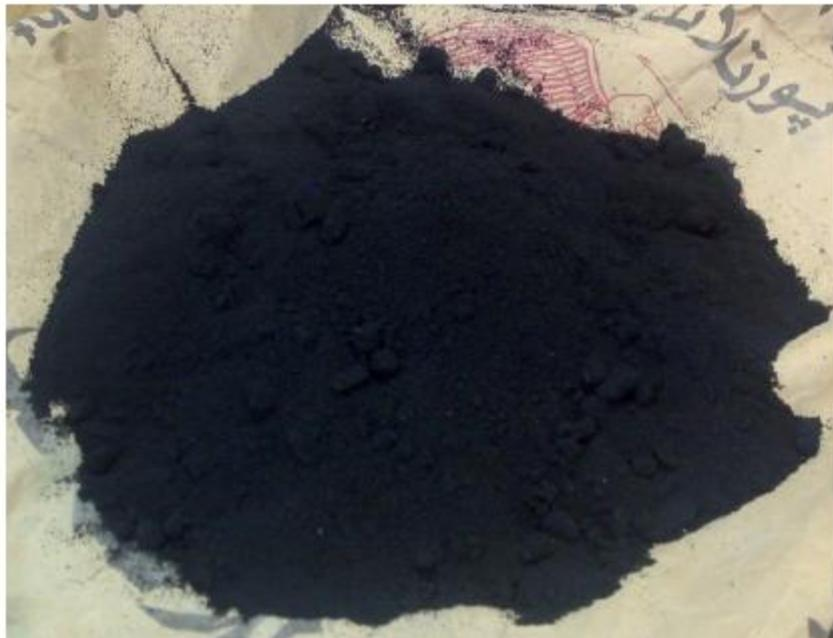
Figure 1: Waste crumb tire rubber [1]
