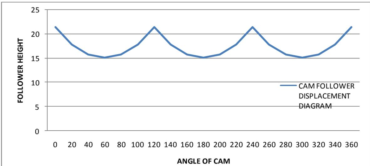
Figure 18. Cam –follower displacement diagram of modified cam.
