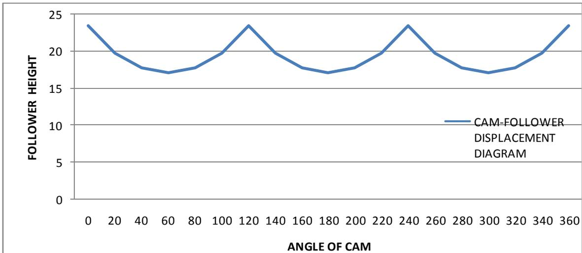
Figure 17. Cam –follower displacement diagram of existing cam.
