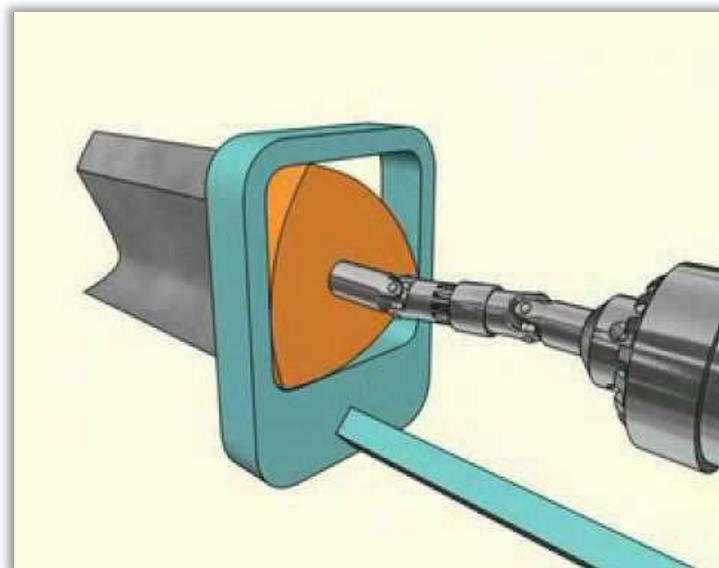
*Figure 3 Square hole drilling operation*
