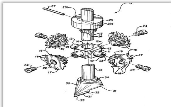
**Figure 4. Reuleaux type drill cutter[5] Figure 5. Disassembled type drill cutter[6]**
