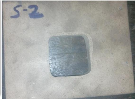
Figure 15. Square hole with modified cam geometry
