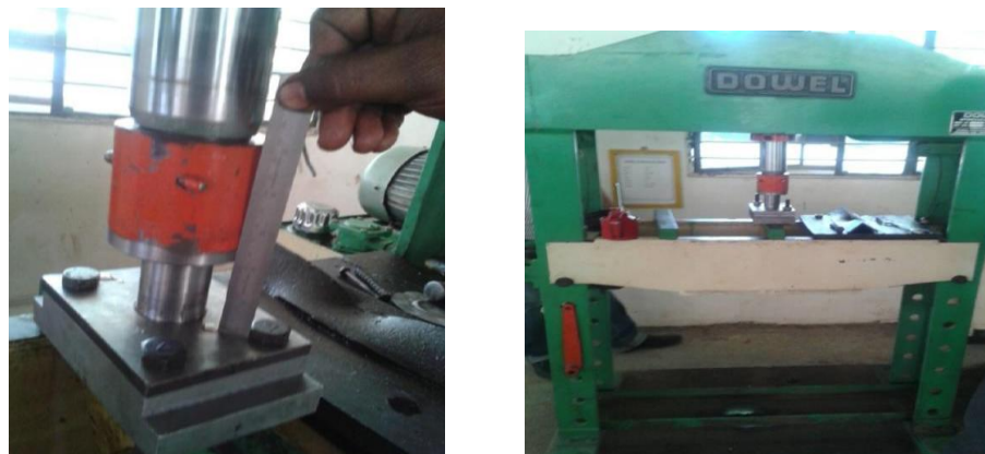
Fig 1.3 Experimental set up for performing Deep Drawing operations
