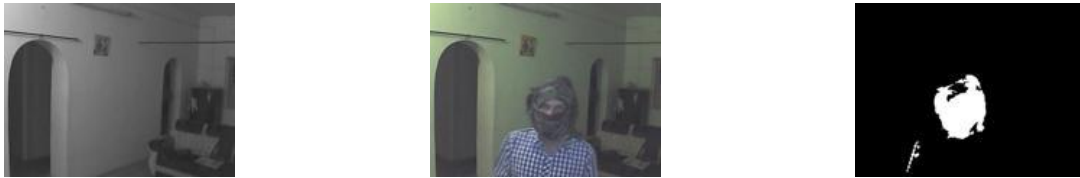
(xviii) (xix) (xx) Figure 10. (xv) – Background Model, (xvi) – Image for processing, (xvii) – Motion detected
