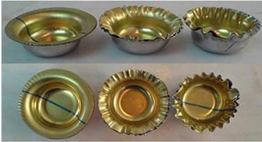
Figure 10: The effect of decreasing the blank holder force (from left to right) on occurrence of wrinkling at the edges of composite blanks.
