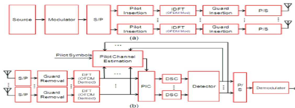
**Fig. 1. Block diagram of the OFDM system, (a): Transmitter, (b): Receiver**
