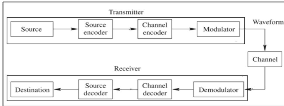
**Figure 1.1: Wireless Communication System**
