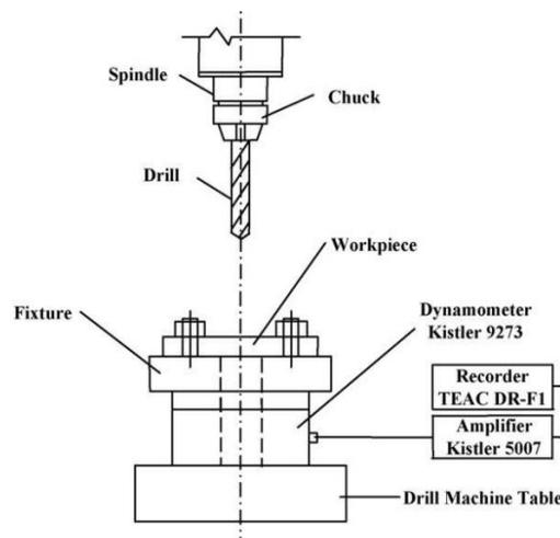
Figure2. Schematic diagram of Experimental Set up.[1]
