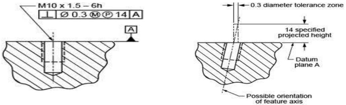
Figure1. Measurement of Perpendicularity.[3]
