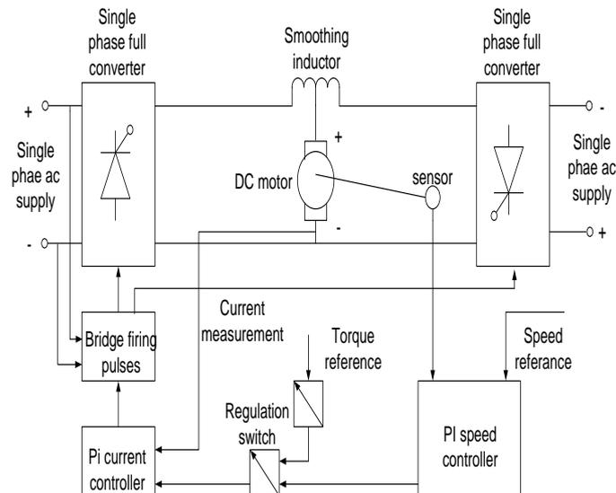
**Figure 2. Schematic block diagram of closed loop dual converter**
