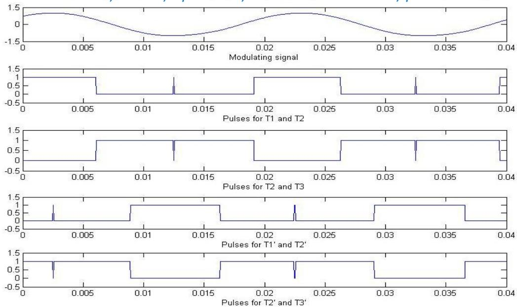
Figure 9 Modulated signal and generated pulses
