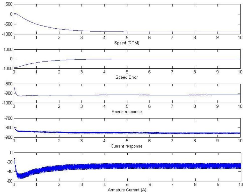
Figure 8.  $W^*=-900$  RPM at  $T=-7.5n.m$  condition Speed, system response and armature current
