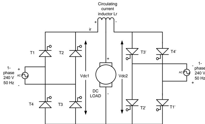
**Figure 1. single phase dual converter with circulating current mode**
