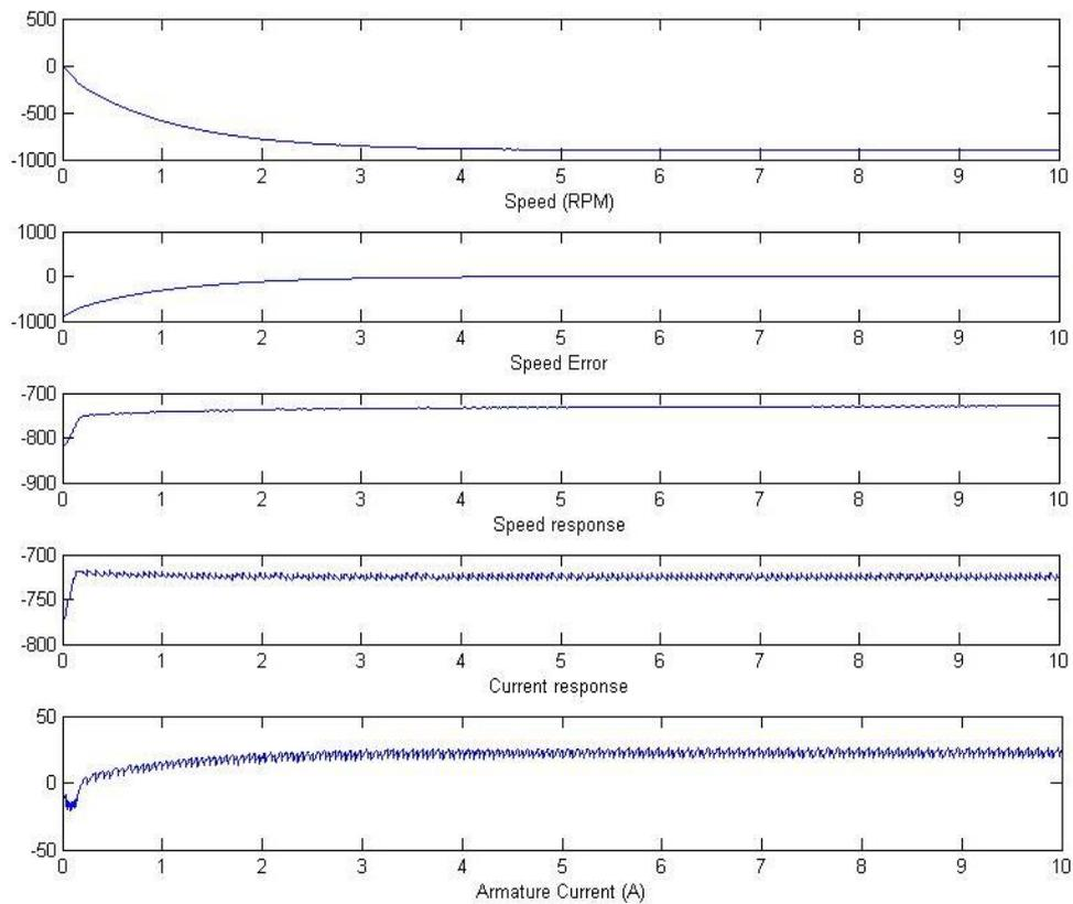
Figure 7.  $W^*=-900$  RPM at  $T=7.5n.m$  condition Speed, system response and armature current
