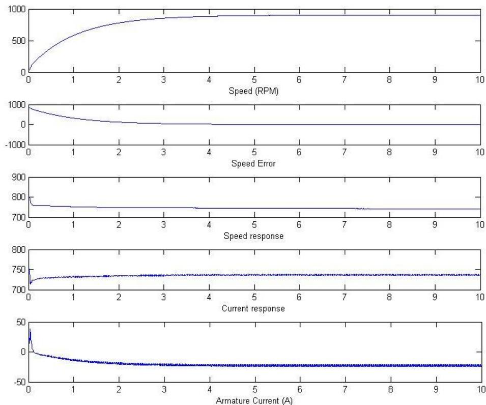
**Figure 6.  $W^*=900$  RPM at  $T=-7.5$  N.m Speed, system response and armature current**
