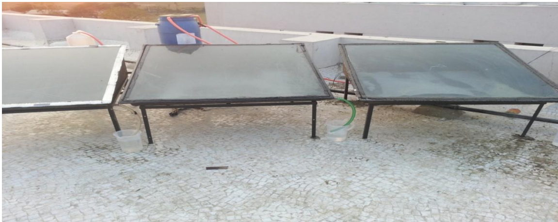
Figure 2 Actual fabrication of solar stills.
