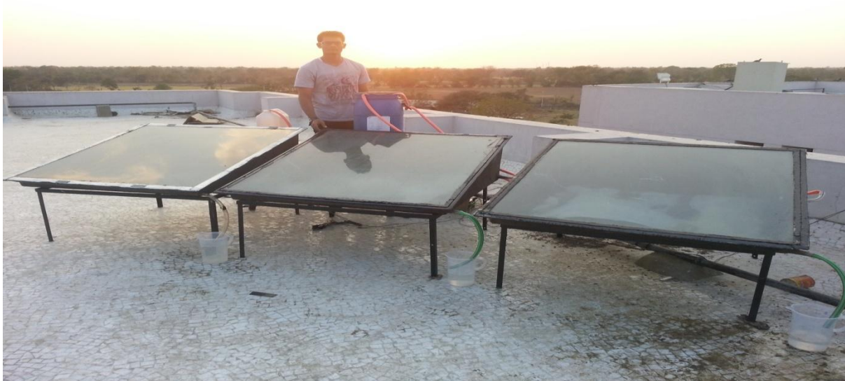
Figure 4 Experimental set up of solar stills.
