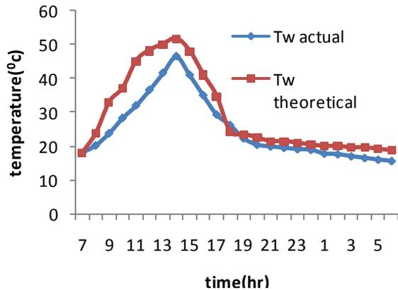
From figure 6 seen that the comparison between actual & theoretical value of glass temperature. So, figure 6 shown that theoretical reading is higher as compared to actual reading. The 18% error is occurred.
