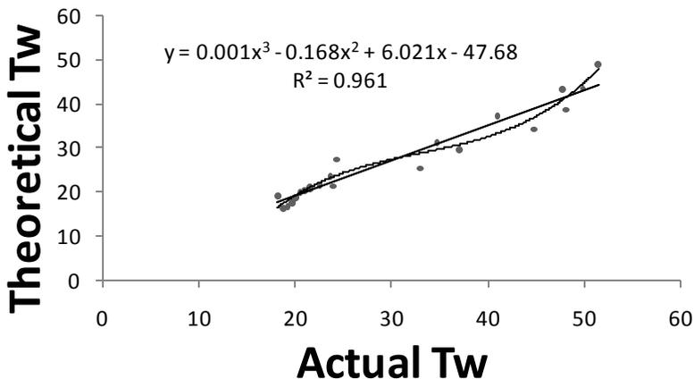
From the figure 5 seen that the comparison between actual & theoretical value of water temperature. So, figure 5 shown that theoretical reading is higher as compared to actual reading. The 14% error is occurred.
