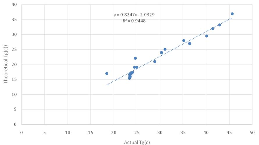
**Figure 8 co-relation between actual & theoretical reading for glass.**
