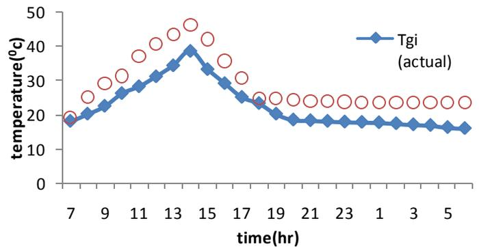
Figure 4 Comparison Of Glass Temperature For Actual & Theoretical (chequered plate)
