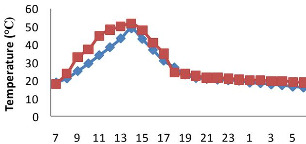
Figure 3 Comparison of Water Temperature for Actual & Theoretical (chequered plate)
