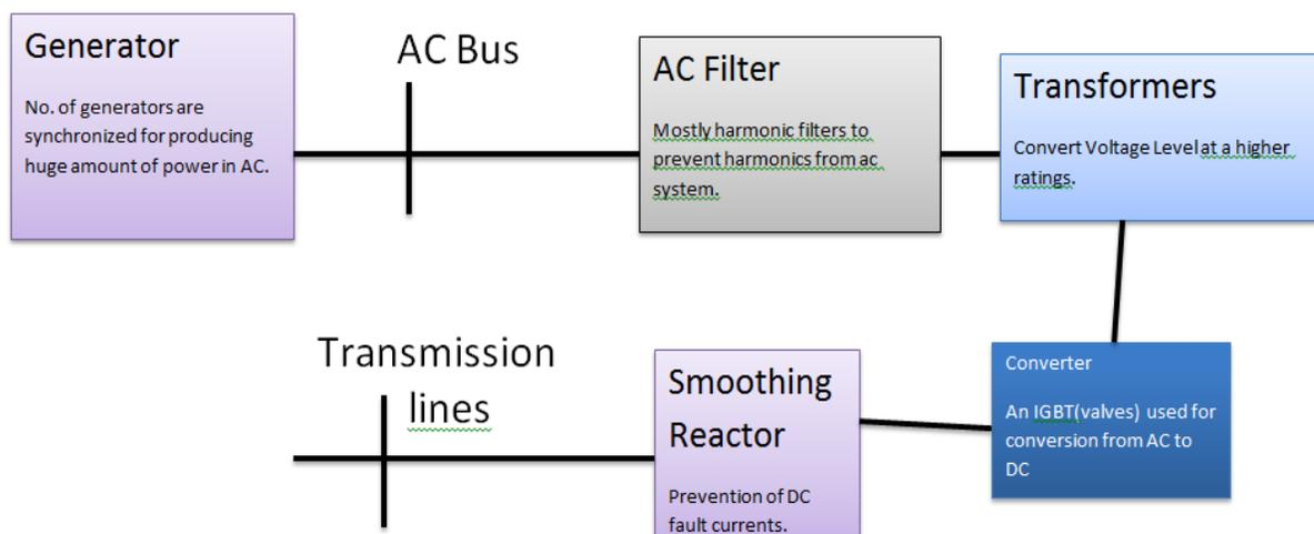
Fig.5 Schematic diagram for HVDC transmission links
