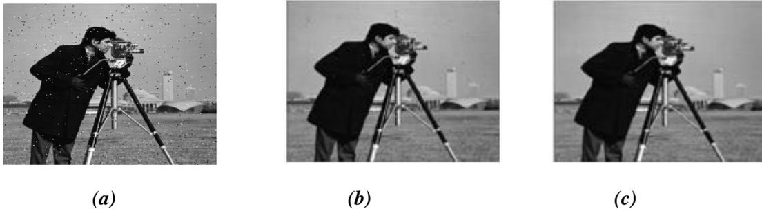
**“Figure 13. (a) Original Image (b), (c) Result of median filter”**
