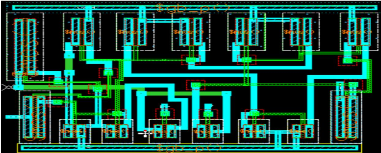
Figure 5: A layout design of class AB variable gain amplifier
