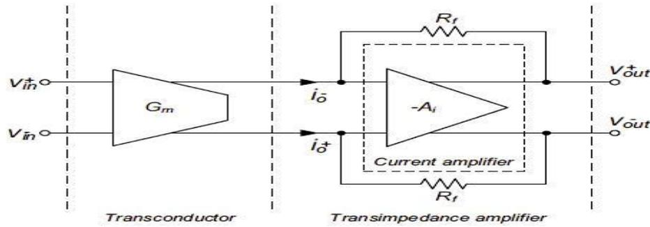
Figure 2: Architecture of the proposed VGA stage in [10].
