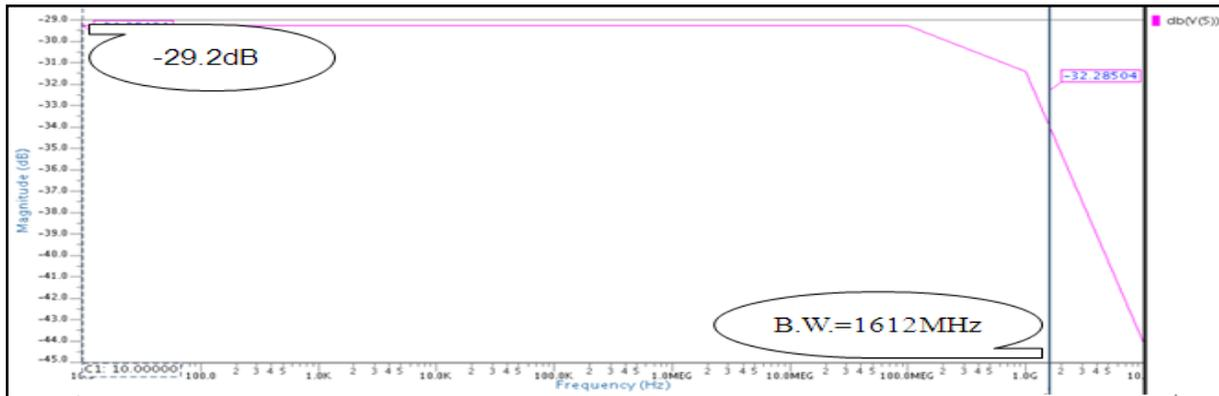
Figure 6:- frequency response at lower gain setting in post-layout simulation
