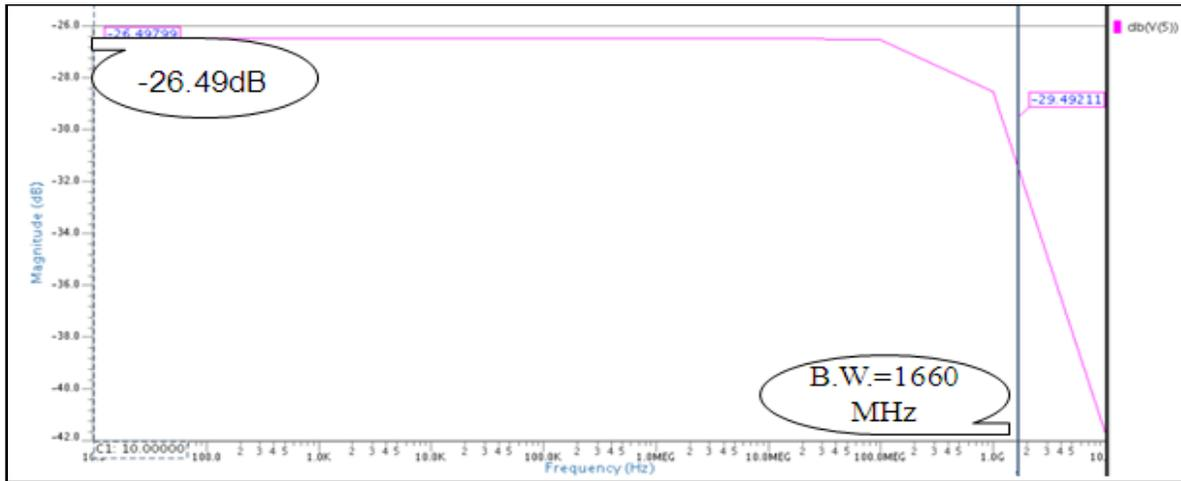
Figure 4:- frequency response at lower gain setting in pre-layout simulation
