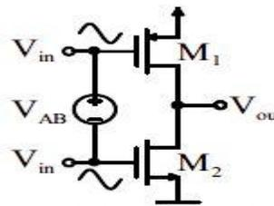
Figure 1: A conceptual common drain stage-based class AB output stage.
