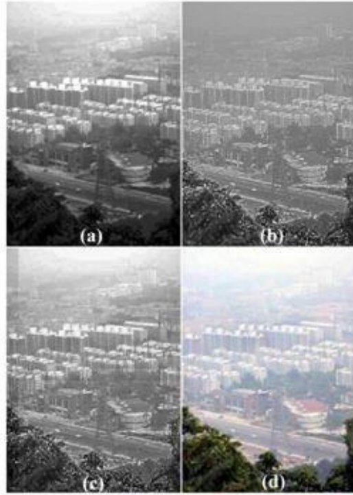
(a) Histogram eq. O/P (b) Sharpening O/P (c) Fusion of Histogram eq. and Sharpening (d) O/P of Prop. method
